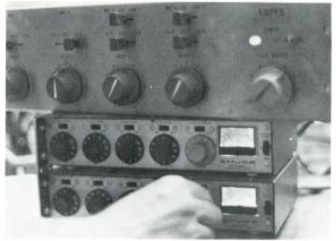
Figure 3. Two Shure M-67's and an Ampex mixer comprise the transportable console.
