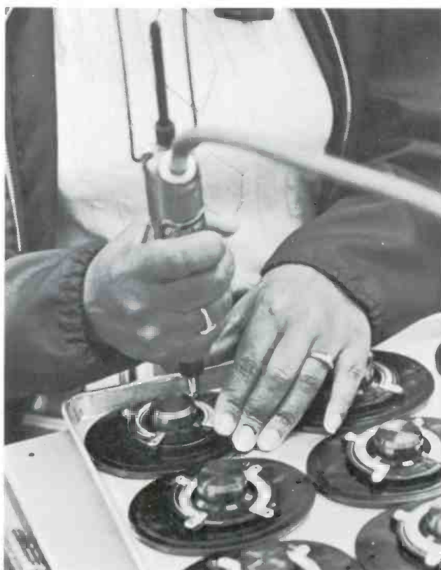
Figure 4. Production of the Pro4 AA elements. Each element is completely manufactured by Koss using specialized machinery developed for this purpose.
